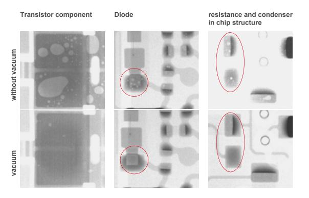
The clearly visible reduction of pore percentage was achieved in the above shown examples via the use of a reflow vacuum soldering system type SMT VAC S.
