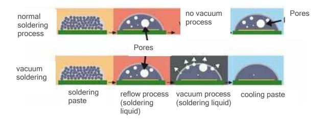
Schematic comparison of conventional (image above "normal soldering process") and vacuum reflow processes (image above "vacuum soldering"). During vacuum reflow processes the vacuum process is programmed as the next step after the actual melting process, which extracts the pores from the liquid solder. This is followed by cooling of the component.
